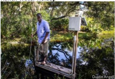
Steffan Pierre on a platform designed to keep his feet dry while performing maintenance on NE-PES monitoring equipment.
